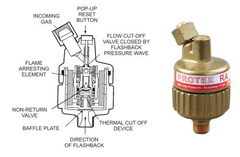
In view of the fact that flashback can occur in any of the cylinders ESAB PROTEX comes in two versions
